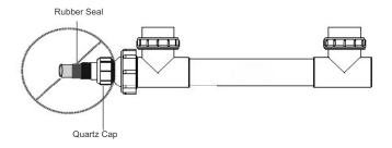
Incorrect: Quartz Sleeve Not Seated See Page 13 for Proper Quartz Sleeve installation
