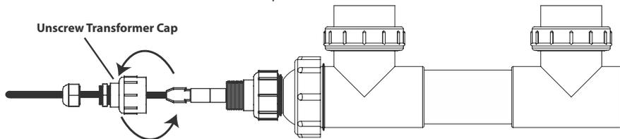
4. Slide Lamp out, be careful not to slide the Lamp out at an angle, even a slight angle, this may cause a “U” shaped crack at the end of the Quartz Sleeve, or possible breakage of the Lamp. Set the lamp on a secure level surface to avoid breakage.
