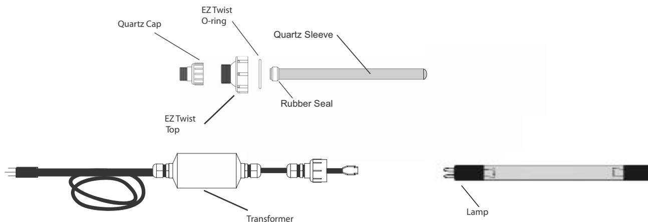
Option 2: If you are not flowing water through your system, drain the unit completely and take the internal parts inside. If the unit is not completely drained, the water will freeze and crack the housing. This is not covered under warranty.
