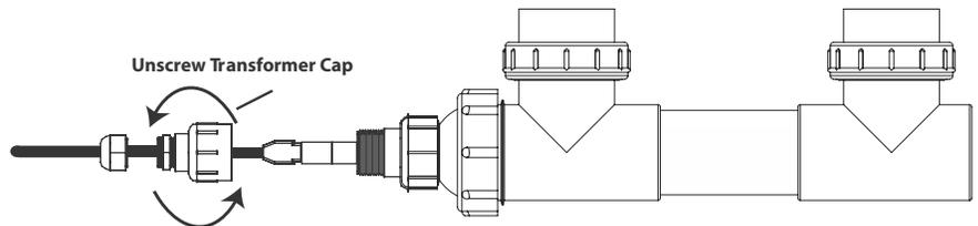
4. Slide Lamp out, be careful not to slide the Lamp out at an angle, even a slight angle, this may cause a "U" shaped crack at the end of the Quartz Sleeve, or possible breakage of the Lamp. A Broken Lamp or Quartz Sleeve is not covered under warranty.
