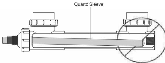
Incorrect: Lamp at an Angle will create a U Shaped Crack
