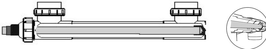
6. Gently push the Quartz Sleeve and Rubber Seal in to the E-Z Twist Top until only ½ of the rubber seal is visible.
