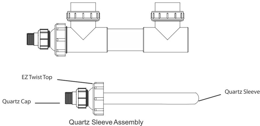
2. Untwist E-Z Twist Top. This will release the Quartz Sleeve Assembly. Pull The Quartz Sleeve Assembly straight out of the housing.
