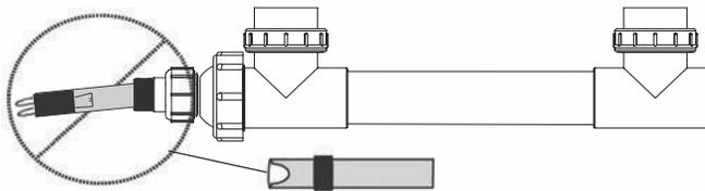
Incorrect: Lamp Not Plugged Flush with Lamp End Connector
