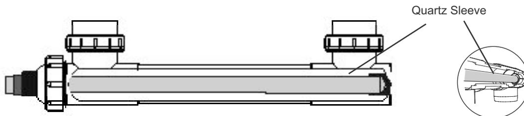
8. Screw on the E-Z Twist Top. Do not use a pipe wrench, pliers or any other tool on this unit. Tighten by hand only. Re-install the Lamp as Shown on page 19, starting at #6.
