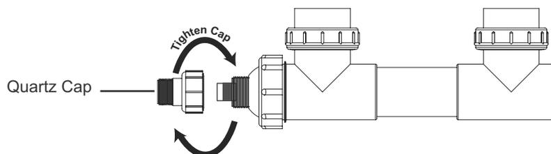
7. Twist on the Quartz Cap. DO NOT use a pipe wrench, pliers or any other tool on this unit. Tighten by hand only.
