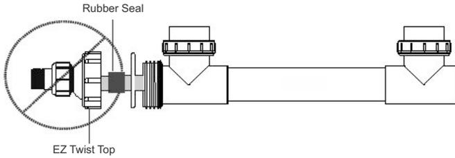
Incorrect: Rubber Seal is Outside of Quartz Cap
