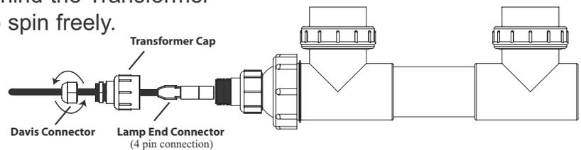
2. Plug the Lamp flush into the Lamp End Connector before inserting the Lamp into the unit. If the Lamp is not plugged in all the way it may cause damage to the unit which is not covered under warranty.
